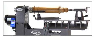
Position the gap at the end of the bed to turn long spindles. Note: the banjo bridges the gap.
